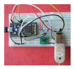
The purpose of this lab is to build and demo several types of widely used I/O interfaces to a small microcontroller. Since this lab uses several input devices in your kit, it would be helpful to read and/or review the wiki page on common user input devices at: https://developer.mbed.org/users/4180 1/notebook/user-input-devices/
