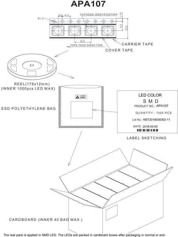
electrostatic bags. cardboard boxes will be used to protect the LEDs from mechanical shocks during transportation. The boxes are not water resistant and therefore must be kept away from water and moisture.
