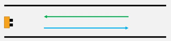
The sonar would be mounted on the wall at the end of a hallway and count how many individuals are walking towards it and away from it
