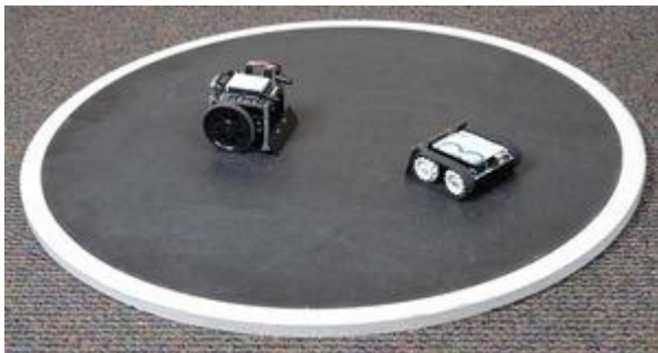
Figure 7 A Zumo Robot in a test arena for evaluating movement and IR sensors [31]
