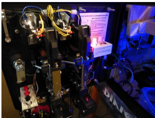
Left: the inside of the coin door. My added service buttons are in the bright cluster in the upper right. This space is normally reserved for a dollar bill acceptor, which I have no need for. Right: a close-up of my custom buttons. The middle button, glowing blue, is the plunger calibration button.
