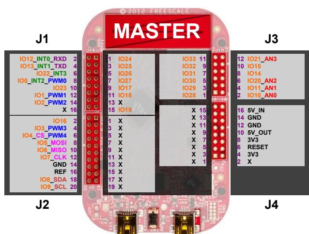
No KE04Z; KL02Z, KL03Z, KL05Z, Arduino do not connect to odd pins
