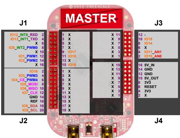
KL02Z, KL03Z, KL05Z, Arduino do not connect to odd pins
