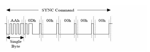
Diagram 2: RS232 SYNC Command Timing SYNC
