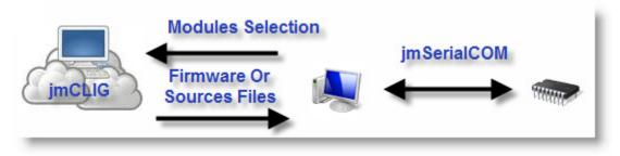
Use standard PC resources and integrated connectivity of the chip to download firmware into it, and control it from a PC.
