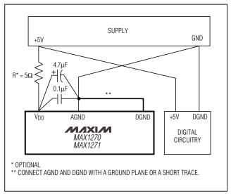
Figure 15. Power-Supply Grounding Connections
