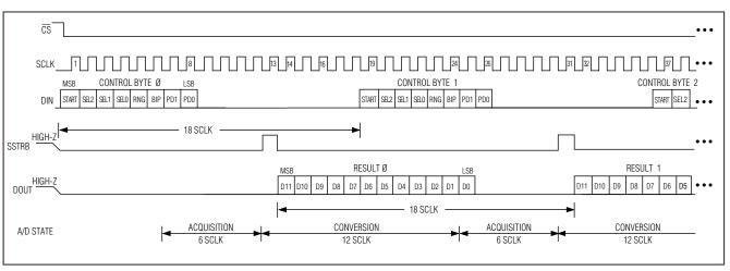
Figure 8. External Clock Mode, 18 Clocks/Conversion Timing
