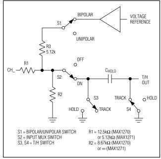
Figure 4. Equivalent Input Circuit
