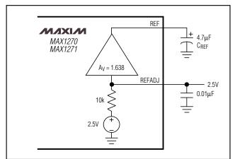
Figure 13c. External Reference, Reference at REFADJ
