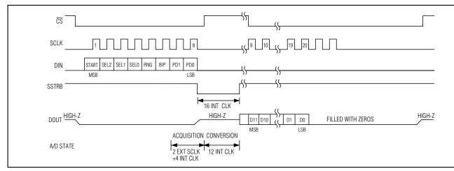
Figure 9. Internal Clock Mode, 20 SCLK/Conversion Timing
