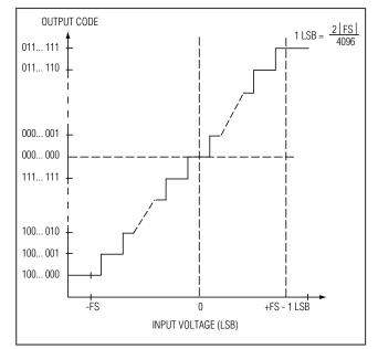
Figure 14b. Bipolar Transfer Function
