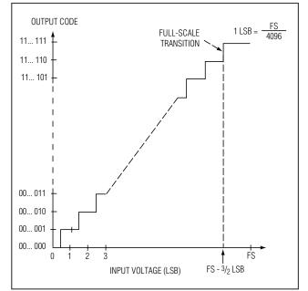
Figure 14a. Unipolar Transfer Function
