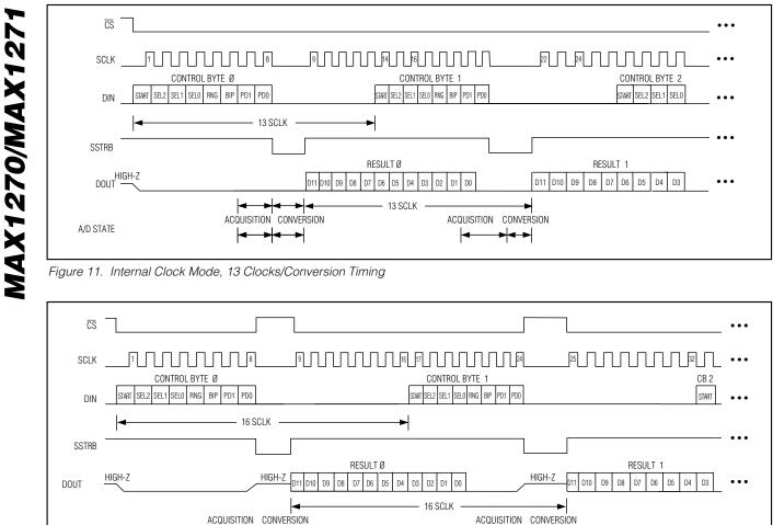
Figure 12. Internal Clock Mode, 16 Clocks/Conversion Timing
