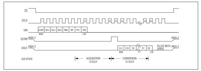
Figure 6. External Clock Mode, 25 Clocks/Conversion Timing
