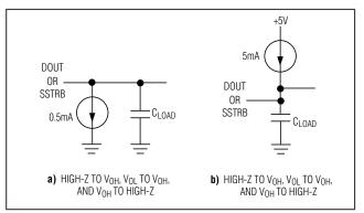
Figure 2. Output Load Circuit for Timing Characteristics
