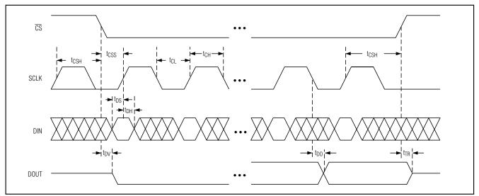
Figure 5. Detailed Serial-Interface Timing
