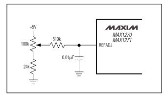
Figure 1. Reference-Adjust Circuit
