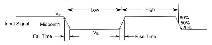
The midpoint is  $V_{IL}$  + ( $V_{IH}$  -  $V_{IL}$ ) / 2
