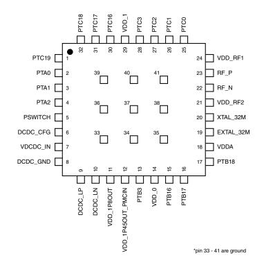
Figure 18. 32-pin Laminate QFN pinout diagram
