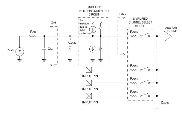
Figure 7. ADC input impedance equivalency diagram
