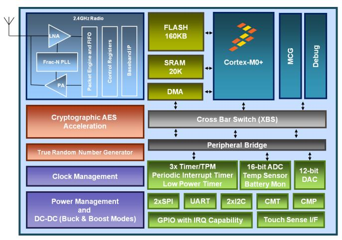
Figure 1. KW40Z/KW30Z/KW20Z simplified block diagram
