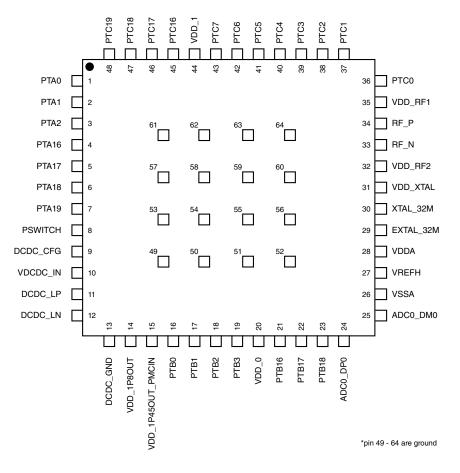
Figure 17. 48-pin Laminate QFN pinout diagram
