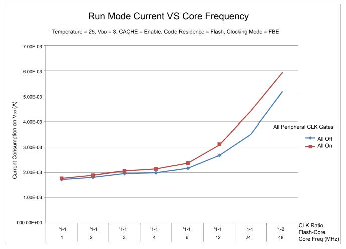
Figure 3. Run mode supply current vs. core frequency
