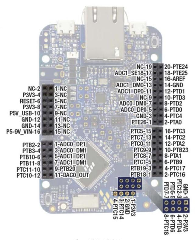
Figure 18. FRDM-K64F pinout
