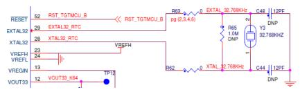
Figure 8. 32.768 KHz crystal for RTC
