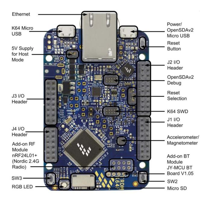
Figure 2. FRDM-K64F main components placement
