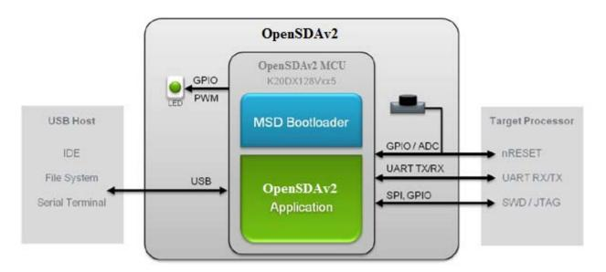
Figure 4. OpenSDAv2 high-level block diagram
