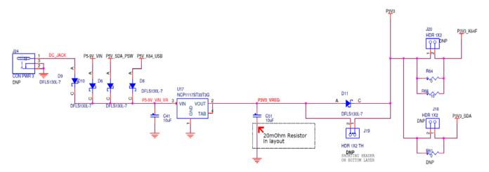
Figure 3. Power supply schematic
