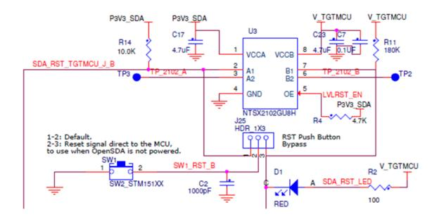
Figure 15. Reset circuit
