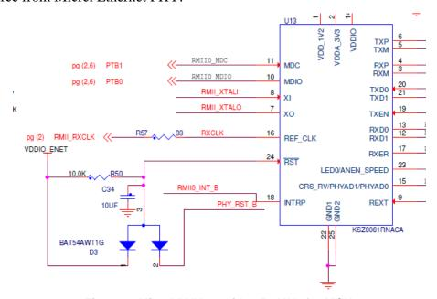
Figure 6. Micrel PHY provides 50 MHz for MCU
