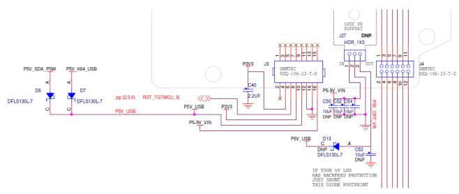
Figure 10. K64 USB power input for host mode
