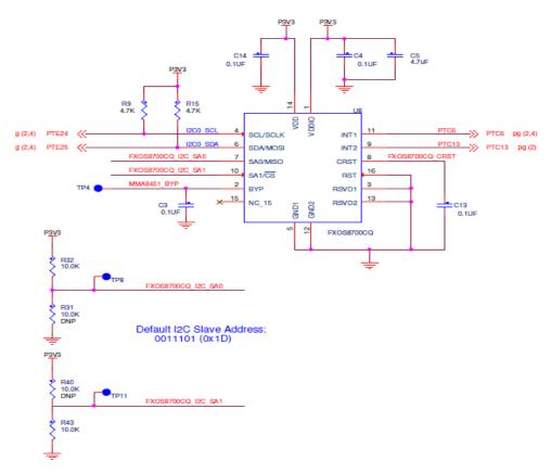
Figure 13. Accelerometer and magnetometer
