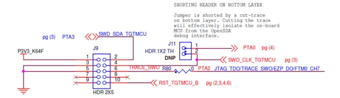
Figure 5. SWD debug connector
