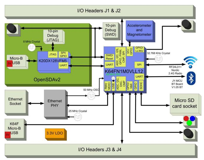
Figure 1. FRDM-K64F block diagram
