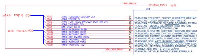
Figure 7. MCU receives RMII clock from Micrel Ethernet PHY
